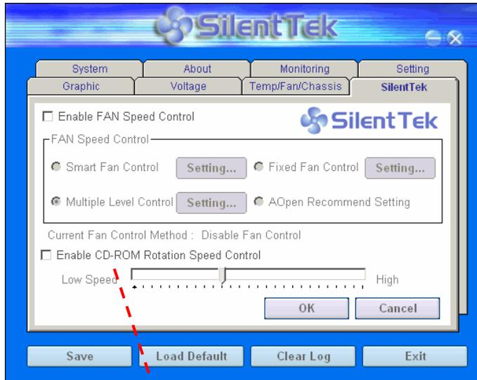
1. **Smart FAN Control:** This is the default setting of SilentTek and can be used for any branded computer housing. With a special algorithm developed by AOpen, the fan speed is automatically adjusted by the factors of CPU and ambient temperature. Ease-of-use and trouble free at your service.
