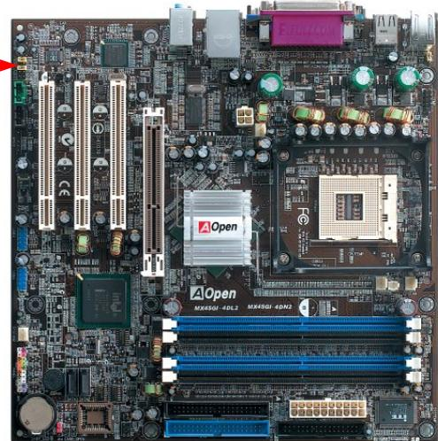
**Note:** Please remove the jumper cap from the front audio connector before you connect the cable. Do not remove this yellow jumper cap if your housing doesn't have an audio port on the front panel.
