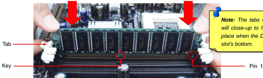
**Note:** The tabs of the DIMM slot will close-up to hold the DIMM in place when the DIMM touches the slot's bottom.
