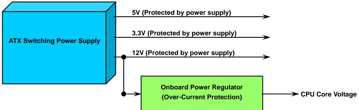
**Note:** Although we have implemented protection circuit try to prevent any human operating mistake, there is still certain risk that CPU, memory, HDD, add-on cards installed on this motherboard may be damaged because of component failure, human operating error or unknown nature reason. **AOpen cannot guaranty the protection circuit will always work perfectly.**
