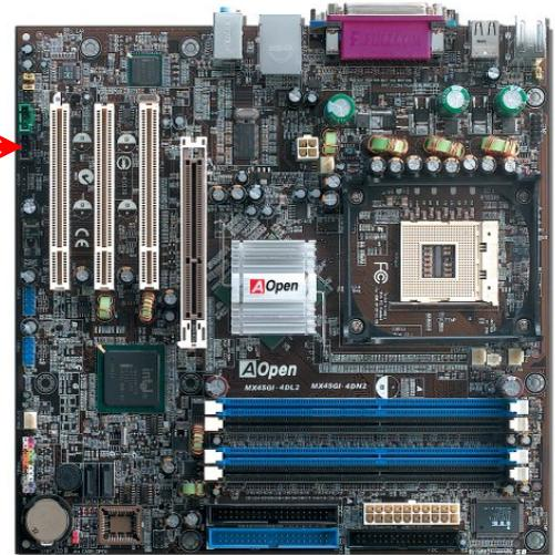
**Note:** Though some of the latest versions of Windows support "Digital Audio" through IDE bus. However, in order to use Open Jukebox player, which is driven under BIOS, it is a **MUST** to connect audio cable to CD-IN connector on the motherboard.
